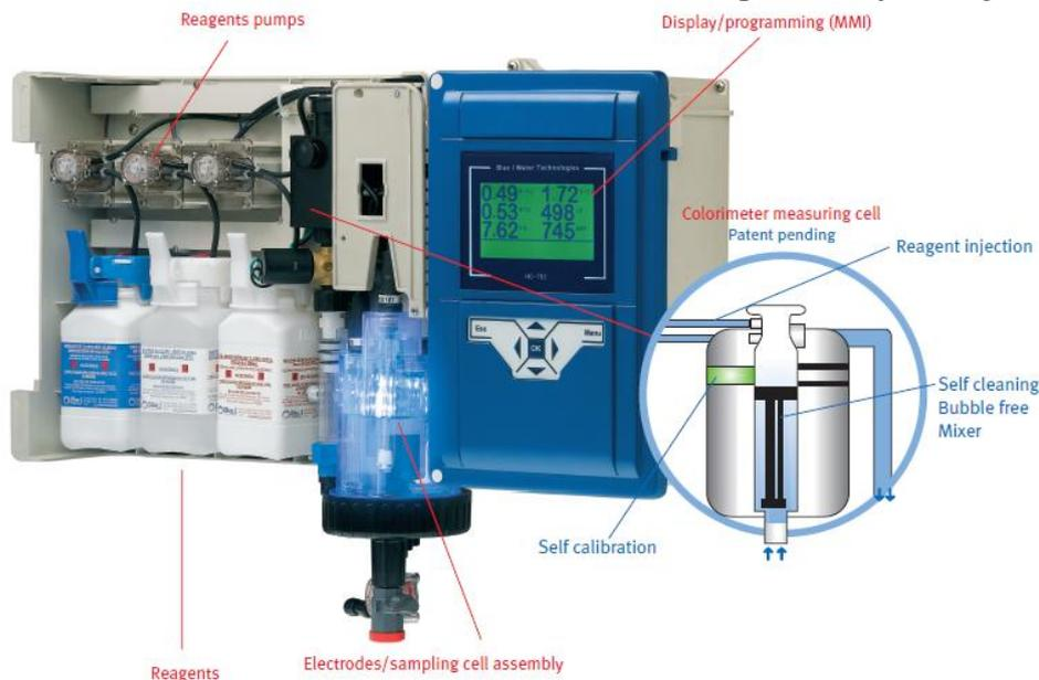
Figure 3: Analyzer schematics
